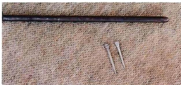
Top: Borium tube, used for welding beads or "cleats" on shoes. Bottom left: Commercially available Borium headed nail. Bottom right: Ordinary horseshoe nail, note the smaller head. Photo by Lee Ziegler
